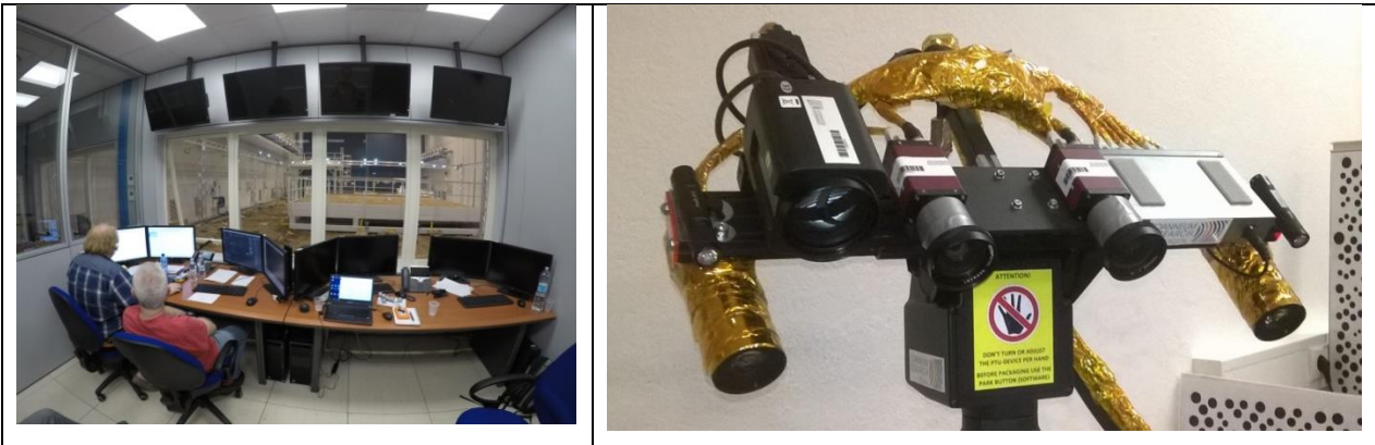
Figure: Left: Control room within the ExoMars ROCC (Rover Operations Control Centre), being the operational environment of NavCam/LocCam 3D vision processing. Right: Geometric PanCam/NavCam Emulator GEPE by JOANNEUM RESEARCH, used for testing and validation of the NavCam/LocCam processing chain.
