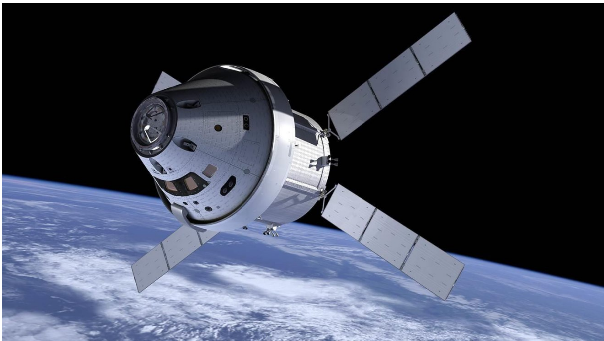
Figure: NASA's Orion spacecraft for providing astronauts into space using a module based on Europe's Automated Transfer Vehicles (ATV). The ATV-derived service module, sitting directly below Orion's crew capsule, will provide propulsion, power, thermal control, as well as supplying water and gas to the astronauts in the habitable module. (Credit: NASA, ESA).
