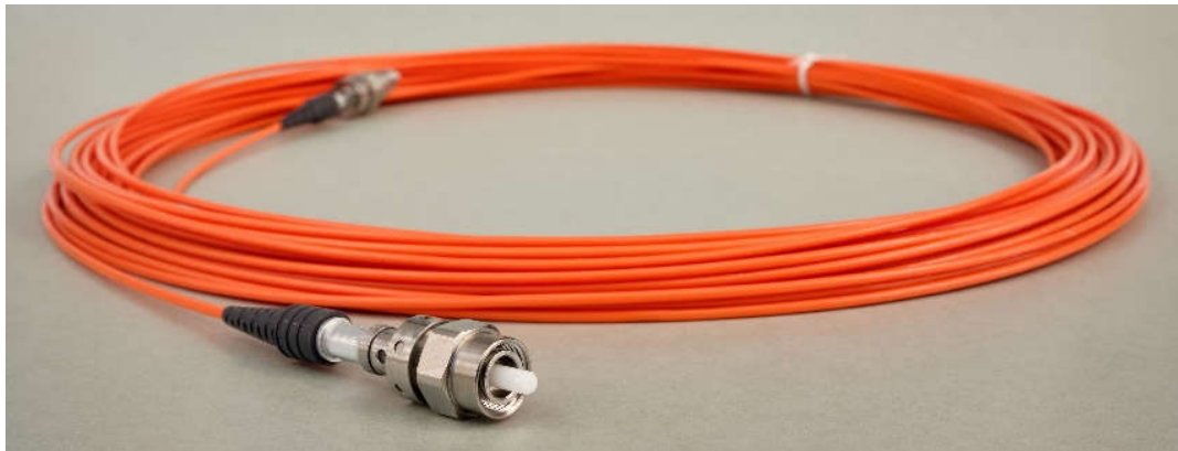
A 400 \mu\text{m} step index multi-mode fiber with non-magnetic connectors and a polymer jacket, which protects the fiber over a wide temperature range from -190\text{ }^{\circ}\text{C} to +120\text{ }^{\circ}\text{C} (© ÖAW/IWF/Pollinger).
