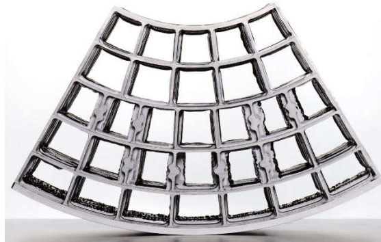
Optical bench demonstrator partly machined (Source: RHP/Robert Syrovatka)
