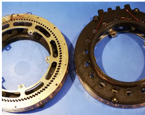
Magnetic Brake: EM during release functional tests at IIES (left) and EM ready for shipping (right)
