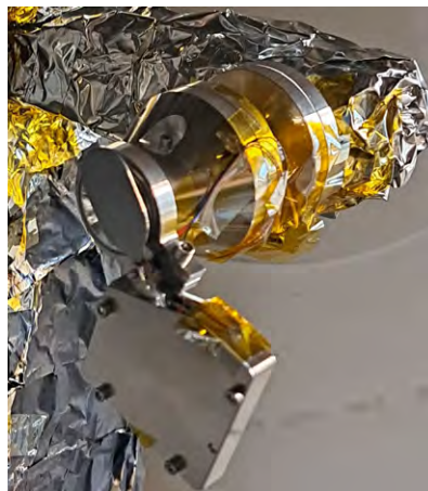
Test setup for characterization of the QCM and validation of the electromagnetic ion shield (left), QCM (middle), electromagnet with collimator (right).
