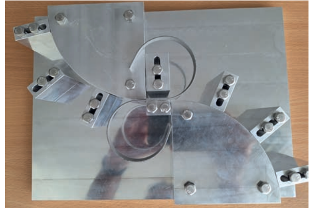
Training setup for the flexible pivot and deployment mechanism made of shape-memory alloy NiTi
