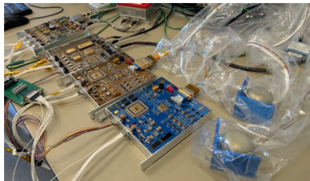
DFP-B2 EFM at integration with two magnetometer boards (blue and brown) in the foreground, data processing unit and power supply in the background and two Engineering Model sensors packed into plastic for contamination protection prepared for thermal vacuum testing. © OeAW/IWF/Valavanoglou
