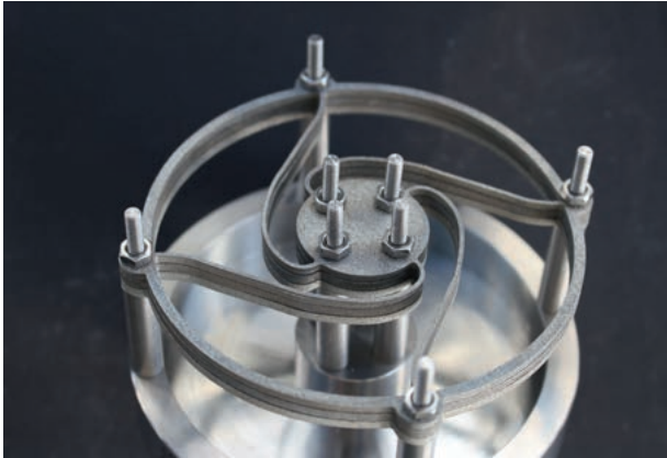
Training setup for the flexible pivot and deployment mechanism made of shape-memory alloy NiTi
