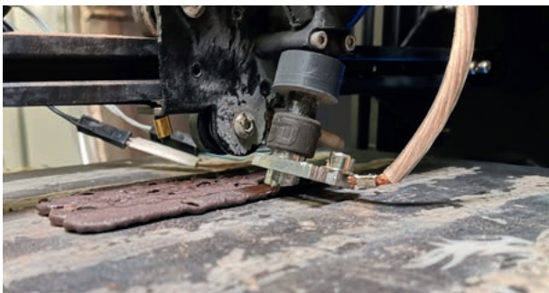
Extrusion-based 3D-printing device processing Martian regolith simulant (left), computer tomography image of 3D-printed regolith sample (right)
