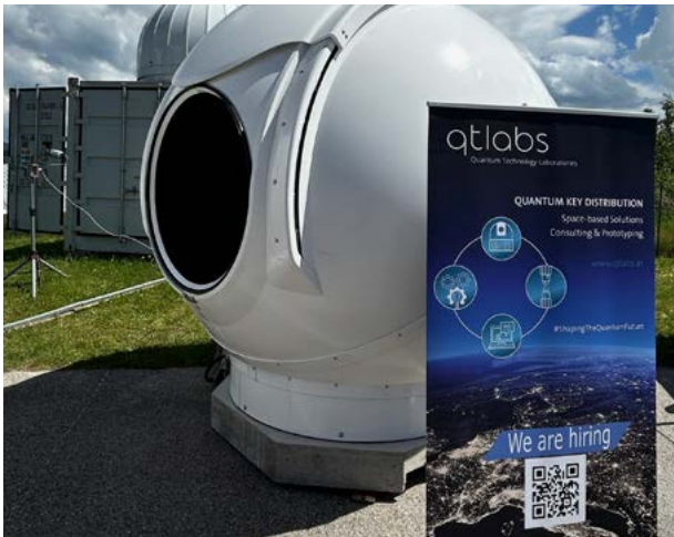
Compact optical ground station with 80cm telescope. © qtlabs
