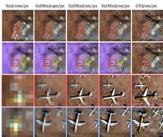
On-board processing: resolution enhancement and target detection. © Fantana GmbH
