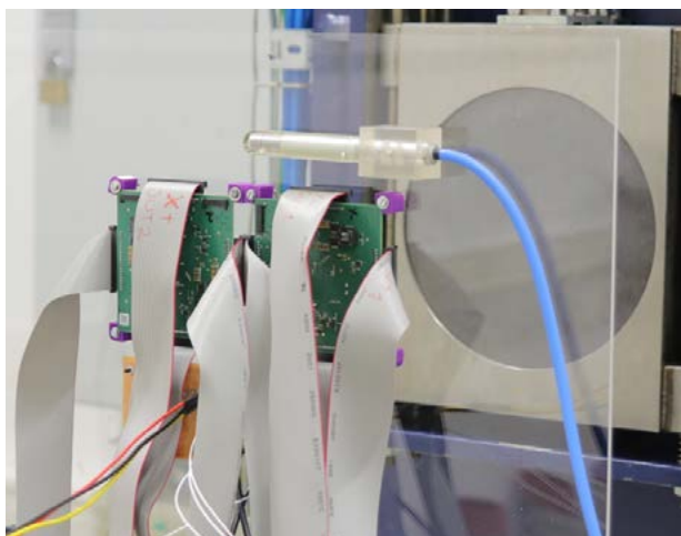
Two CubeSat systems in front of the ^{60}\text{Co} source for exposure to gamma rays during the irradiation test. © FHWN/Seibersdorf Labs
