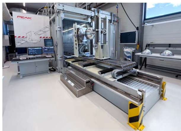
The electron beam welding machine is the newest addition to Peak Technology's expanding production capabilities. © Peak Technology
