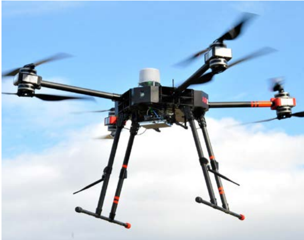
Drone with an onboard satellite terminal © TU Graz
