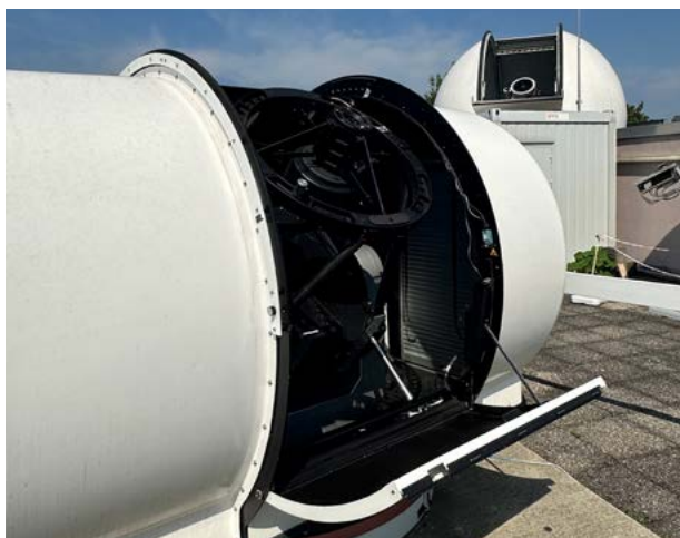
Bistatic MHz space debris laser ranging setup. © ÖAW/IWF
