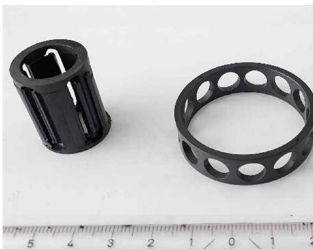
Dry lubrication – cages for different types of bearings © AAC
